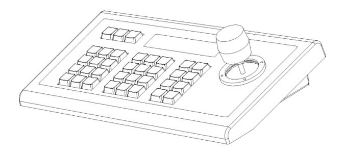
Easy pan, tilt & zoom controls for any RS-232, RS485, RS422 VISCA, Pelco-P or Pelco-D protocol camera!
